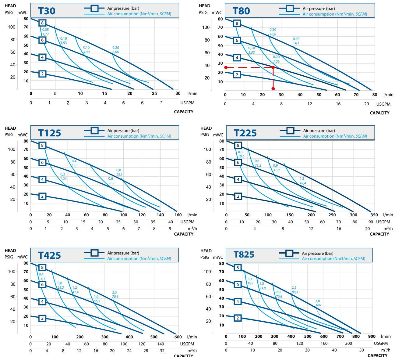
Recommended flow is half of the max flow, i.e. recommended flow for a T80 is 40 l/min (10.6 US gpm).
